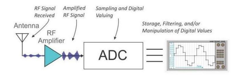
SDR Direct Digital Conversion Receiver Signal Processing
