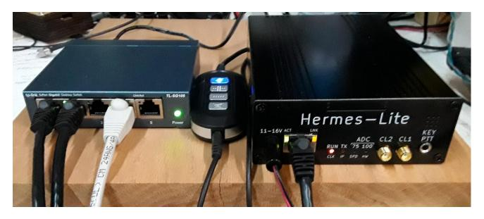
Hermes Lite 2.0 DDC – A Network Based SDR Transceiver Not Homebrew as such; but homebrew units are on the air!
